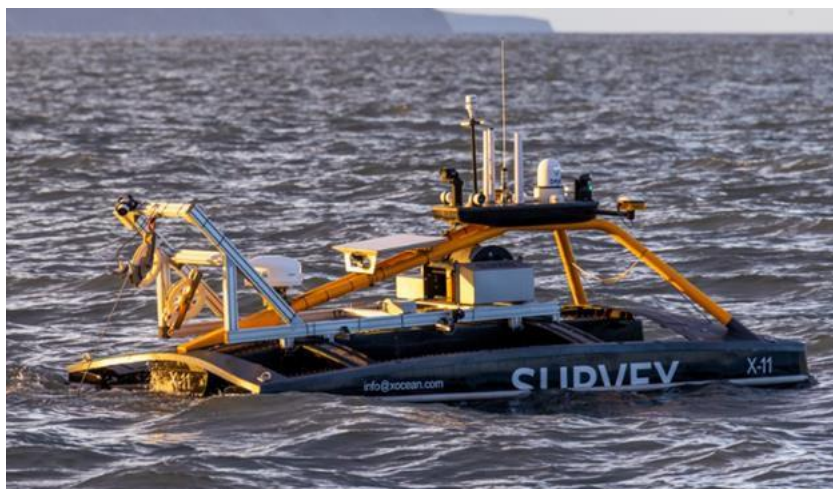
Figure 2: USV with hull mounted sensors
